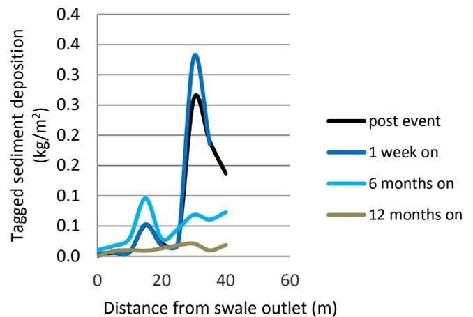
Fig. Deposition of tagged sediment within sediment traps placed in the base of the swale over the 12-month following period
