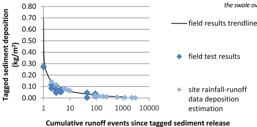
Fig. Trace sediment deposition within the swale over multiple runoff events
