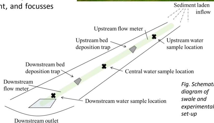
Fig. Schematic diagram of swale and experimental set-up
