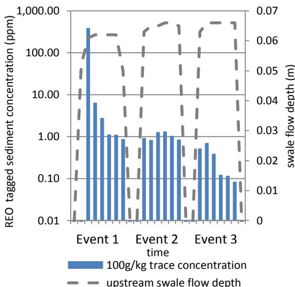
Fig. Flow event suspended sediment transport concentrations
