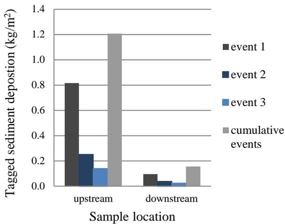
Fig. Deposition of tagged sediment within sediment traps placed in the base of the swale between runoff events
