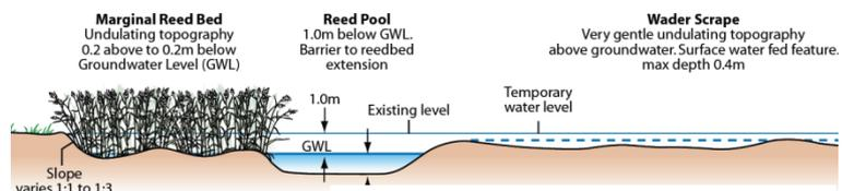
Cross-section (above) showing different approaches to floodplain wetland features: designed for various flood events/ different habitat features.
