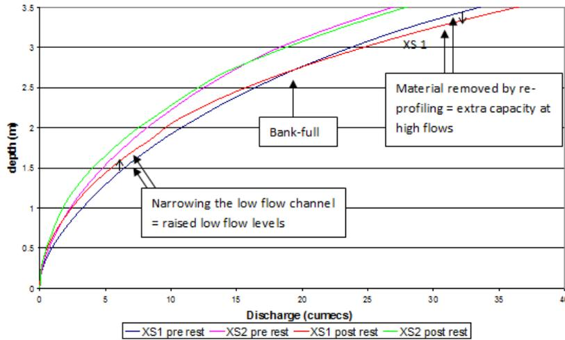
Figure shows an example of where a low flow channel has been dug within a scheme and reprofiling of banks with evidence of change in depth related to discharge.
